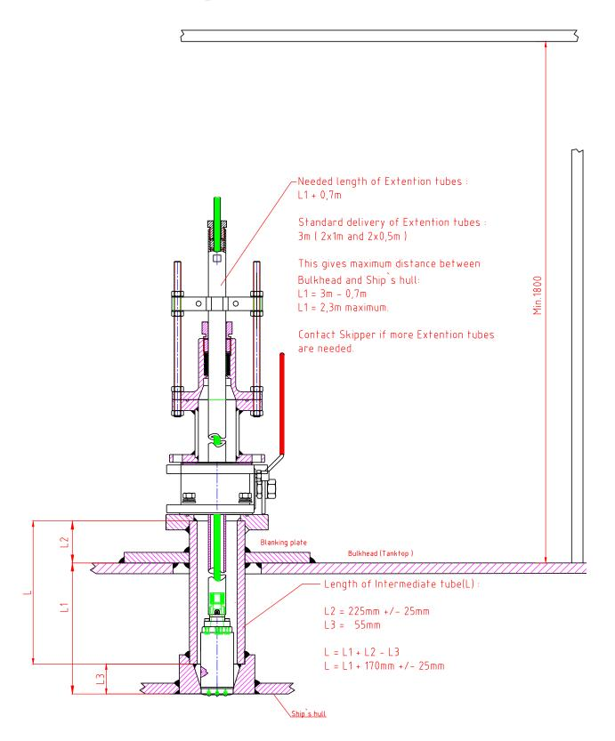
The Ball Valve should be placed in a service accessible place, large enough for installation and disassembly of the sensor unit.
