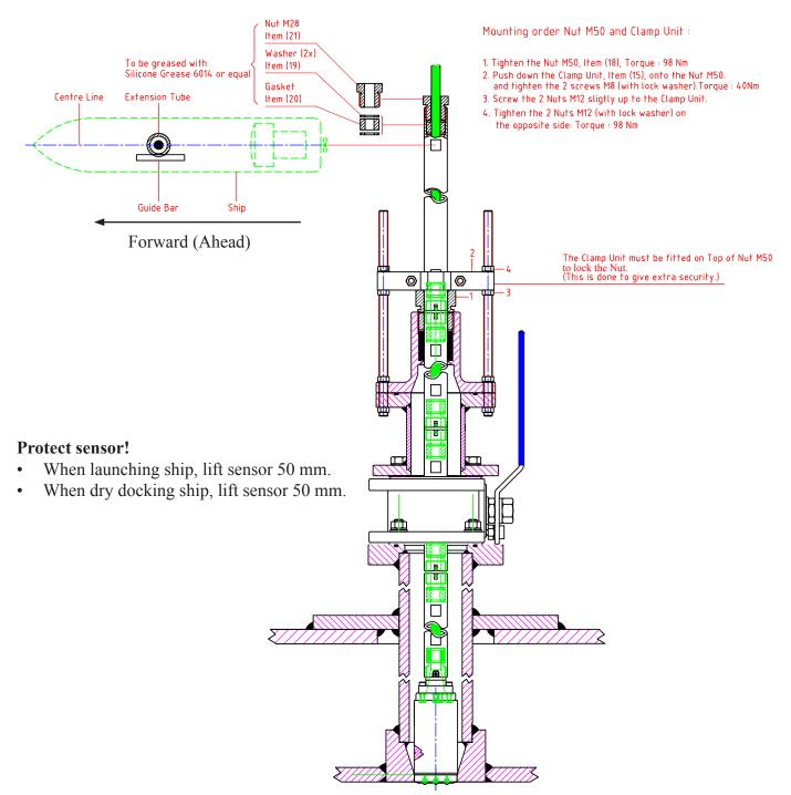
Check that the transducer/sensor housing, when fully inserted, is flush with the lower surface of the bottom flange.
